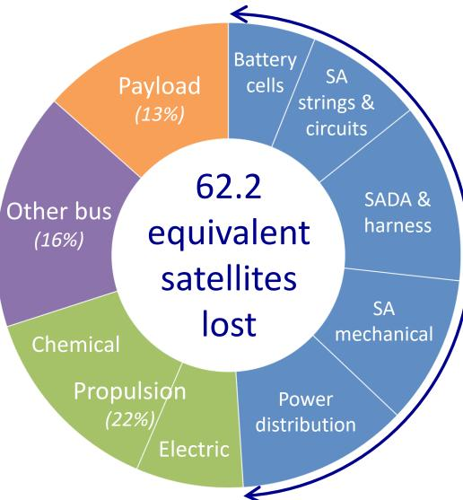
Electrical power subsystem anomalies account for ~50% of loss of capability
